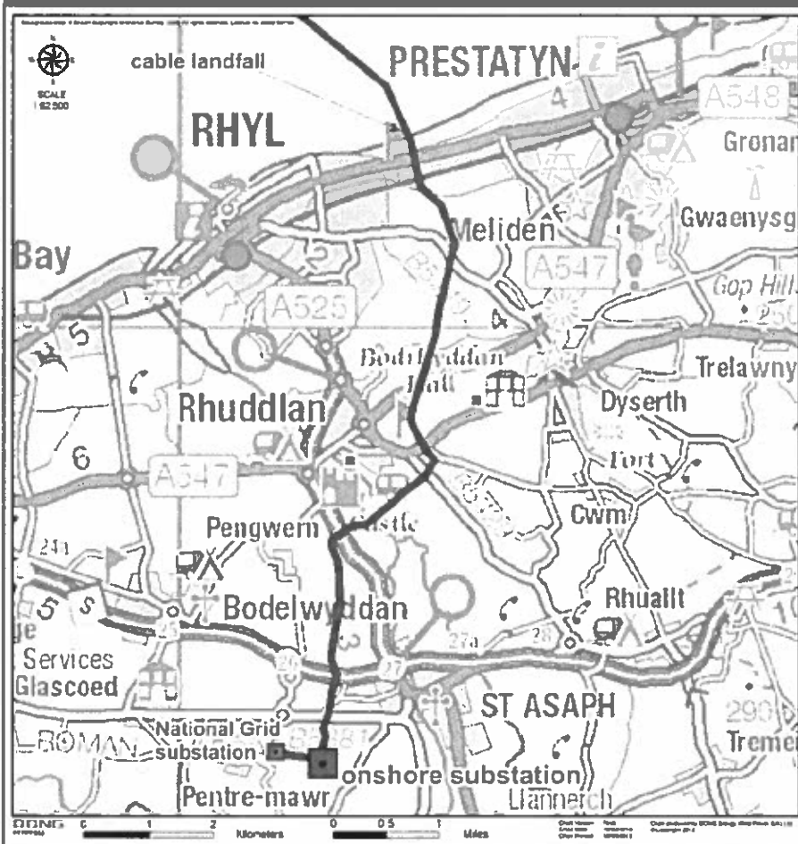
Figure 1.3: Project cable landfall, onshore cable route, substation and National Grid substation, where the energy generated by the Project will ultimately connect
